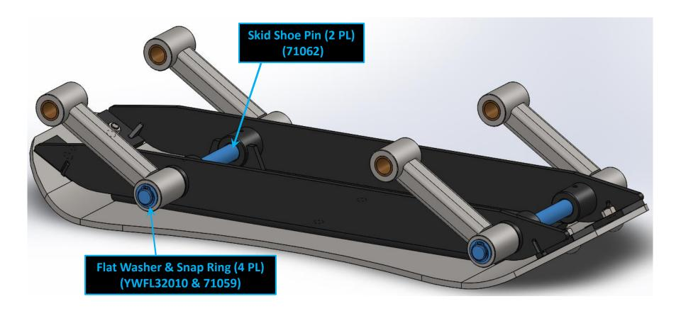
Step 3: Install (1) new Upper Skid Shoe Pins (71062) using (2) Flat Washers (YWFL32010), (2) Snap Rings (71059), and (2) Spacers (71138).
