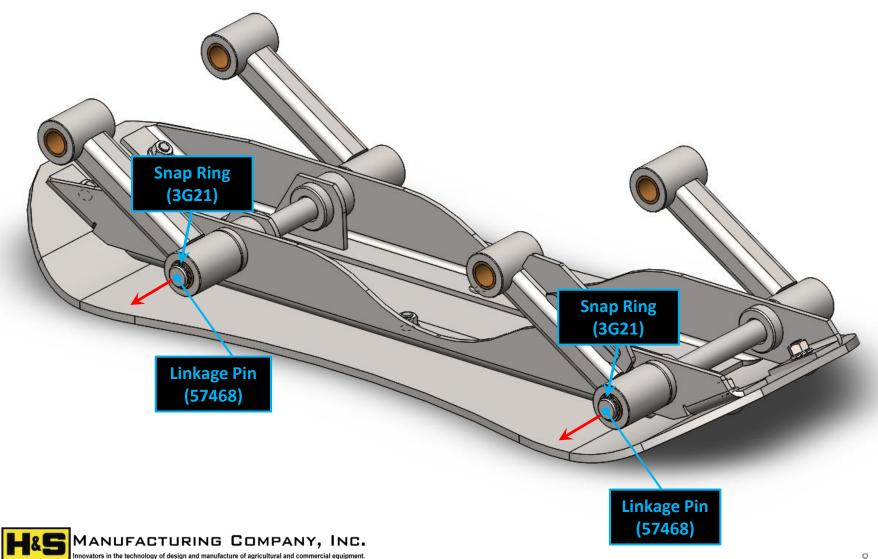
Step 4: Remove (2) existing Skid Shoe Gusset Weldments (63369 & 63370) by removing (4) Carriage Bolts (YBCR16015) and Flange Nuts (YNFG16005) along with (2) Plow Bolts (YBPL16010) and Flange Nuts (YNFG16005). {DISASSEMBLY COMPLETE}
