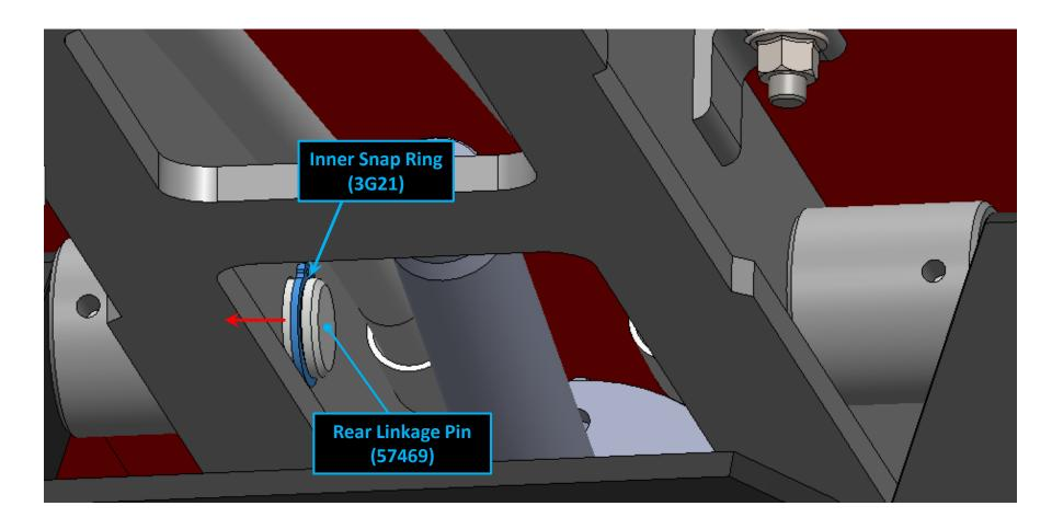
Step 3: Skid Shoe can now be uninstalled from machine. Remove (2) Snap Rings (3G21) to remove the (2) Lower Linkage Pins (57468).
