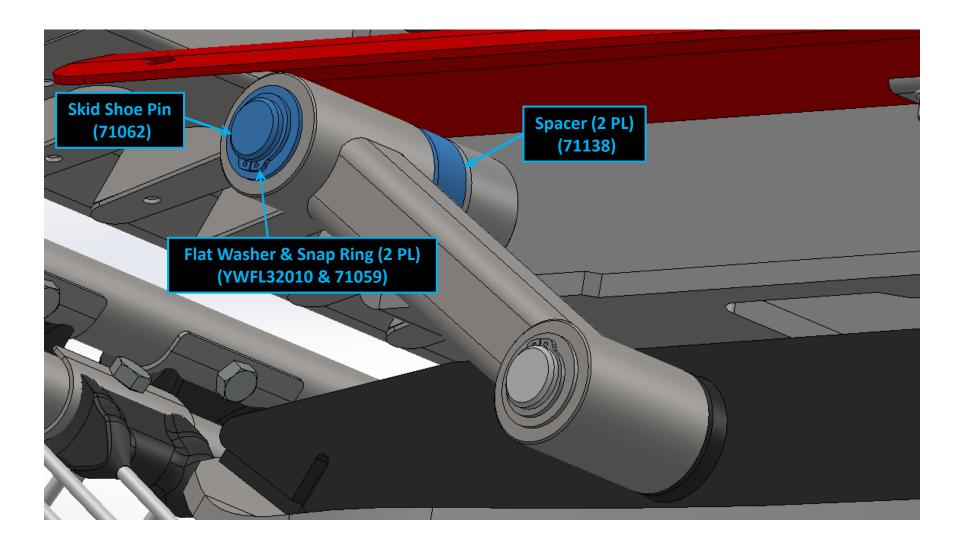
Step 4: Install (2) new Rear Upper Skid Shoe Pins (71058) using (4) Flat Washers (YWFL32010), (4) Snap Rings (71059), and (2) Spacers (71138).
